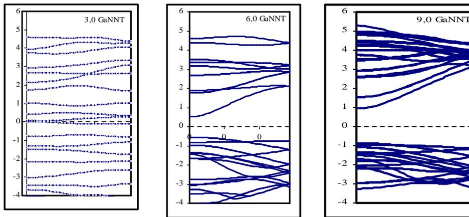
Fig. 1. Band structure of (3,0), (6,0) and (9,0) of GaNNTs.
